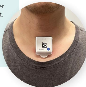
Figure 3: BresoDX1 conveniently attached over the neck to collect tracheal motion and sounds
